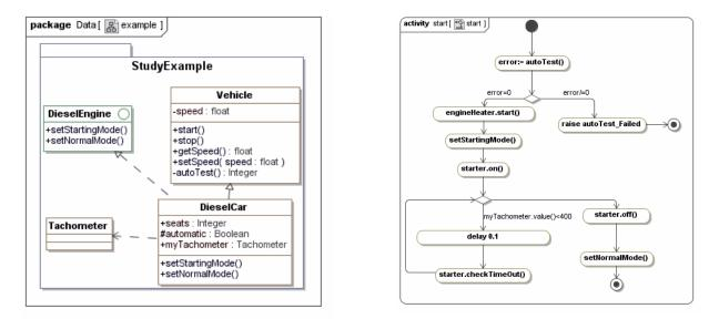
Figure 4. Structural and behavioral models used in the study example.
