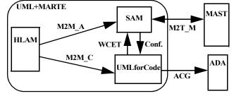
Figure 1. Models & transformations used in this approach
