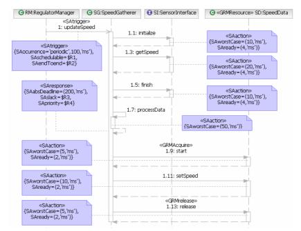
Fig. 3. Sequence Diagram for updateSpeed annotated with the UML profile for SPT
