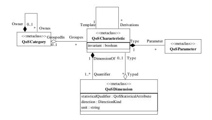
Fig. 4. The QoS Characteristics core model of the UML profile for QoS & FT (Source: [14])
