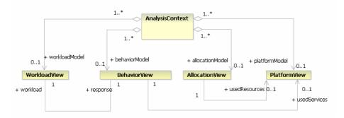
Fig. 10. The Analysis Context model of the QAM Framework
