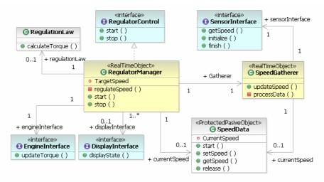
Fig. 2. Structural view for the Speed Regulator example
